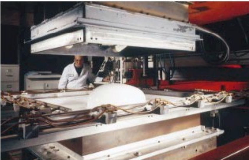
c. Here, the newly formed part is seen cooling on the mold.
