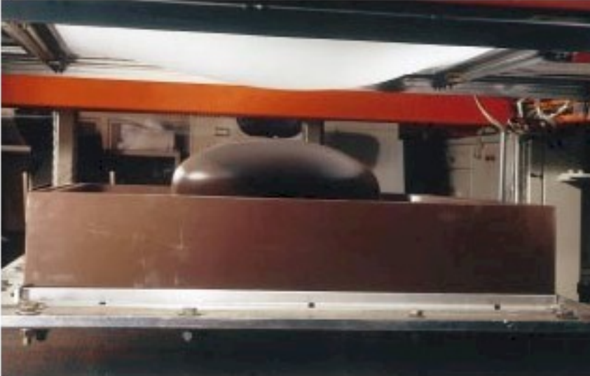
b. After heating in an oven to forming temperature, the sheet is moved into position above the tool.
